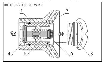
INFLATION MODE: valve is closed with gasket 4 tight. To move the valve to deflation mode: push the button 6 and turn it clockwise to fix it in lower position
